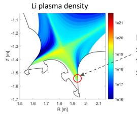
Li emission simulated by puffing from the target with specified flow rate
