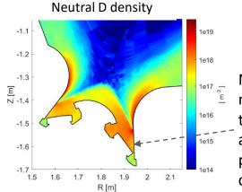
Mesh for kinetic neutrals extends up to physical wall → account for pumping / condensation
