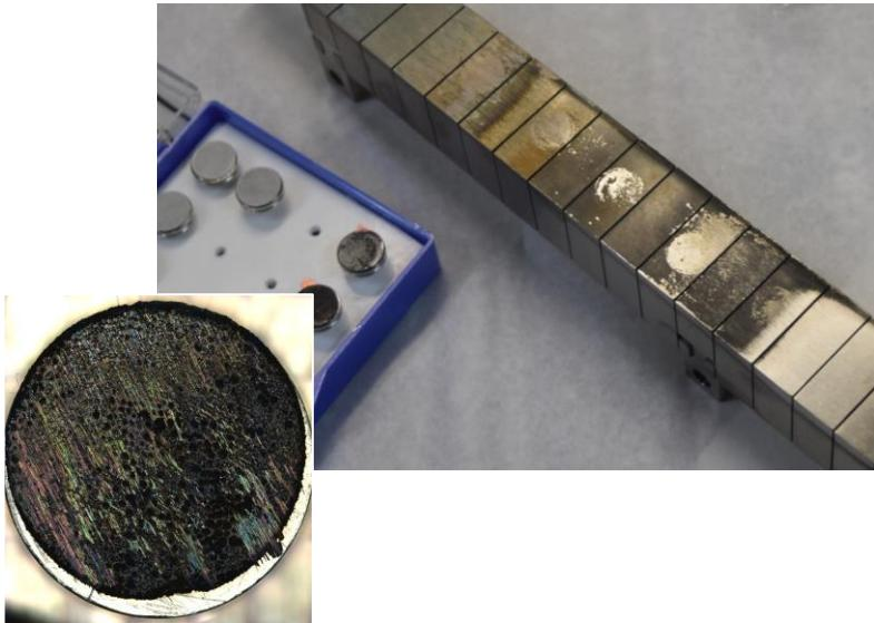
Erosion/Redeposition patterns on the lower divertor sector
