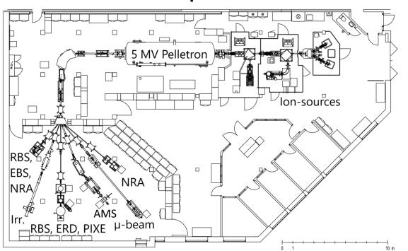
2 gas & 2 sputter ion sources – beams of H, D, <sup>3</sup>He, <sup>4</sup>He, C, N, O, Cu, Br, I, Au, ...
