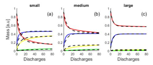
evolution of total in-vessel mobilizable (red), non-mobilizable (blue), splashed (green) and vaporized (yellow) dust mass, for various initial size distributions
