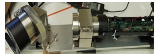
EDICAM wide-angle camera (in commissioning in Naka)
