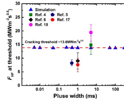
**The Heat Flux factor is independent of pulse duration**
