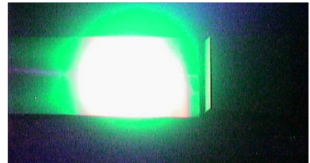
W/ Cu composite, adiabatically loaded above Cu melting
