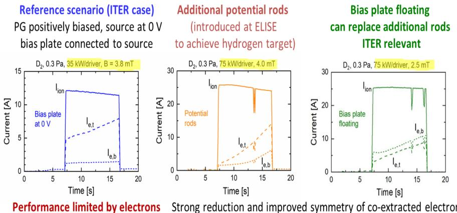
Strong reduction and improved symmetry of co-extracted electrons High power pulses possible -> long pulses will be tested next
