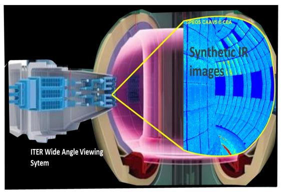
Light propagation in 3D model based on **Monte Carlo Ray Tracing (MCRT) code** (ANSYS-SPEOS CAAV5 here) getting all radiations of thermal scene
