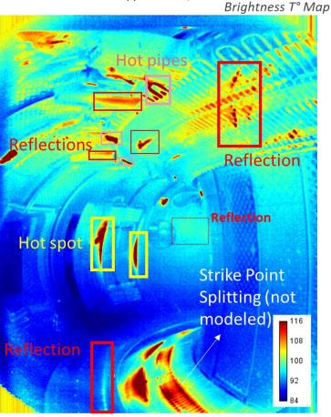
**Experimental IR Image** #Pulse 55210 @ 7s(Ip=500 kA, 4.4MW LH + 0.7MW FCI Brightness T° Map
