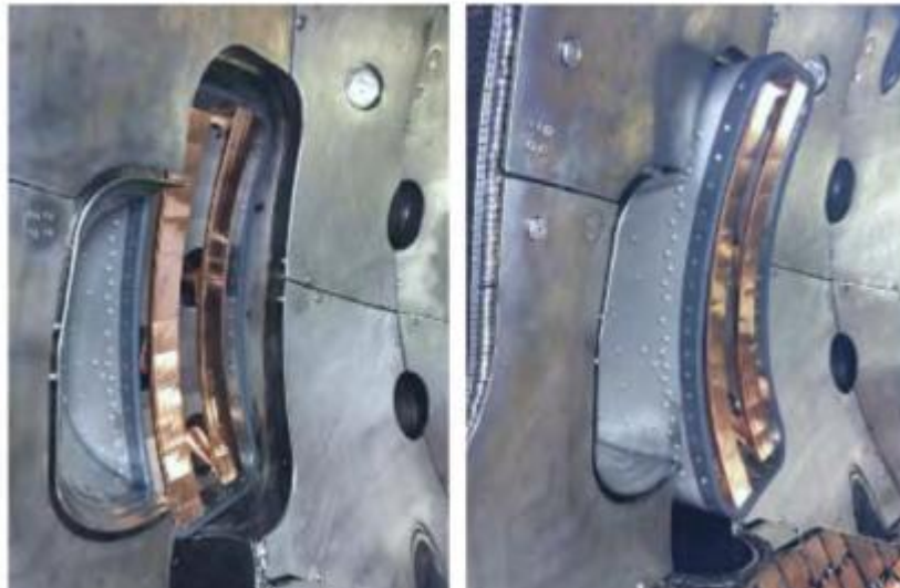
ICRH antenna inside the W7-X plasma vessel
