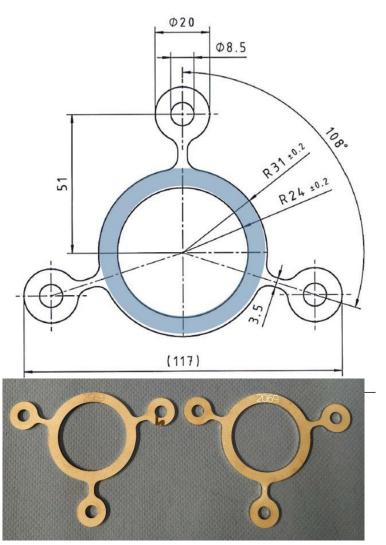
\*Coating thickness: 1 Ring x 150 µm Al 2 O 3 /TiO 2 87/13 1 Ring x 300 µm Al 2 O 3 /TiO 2 87/13
