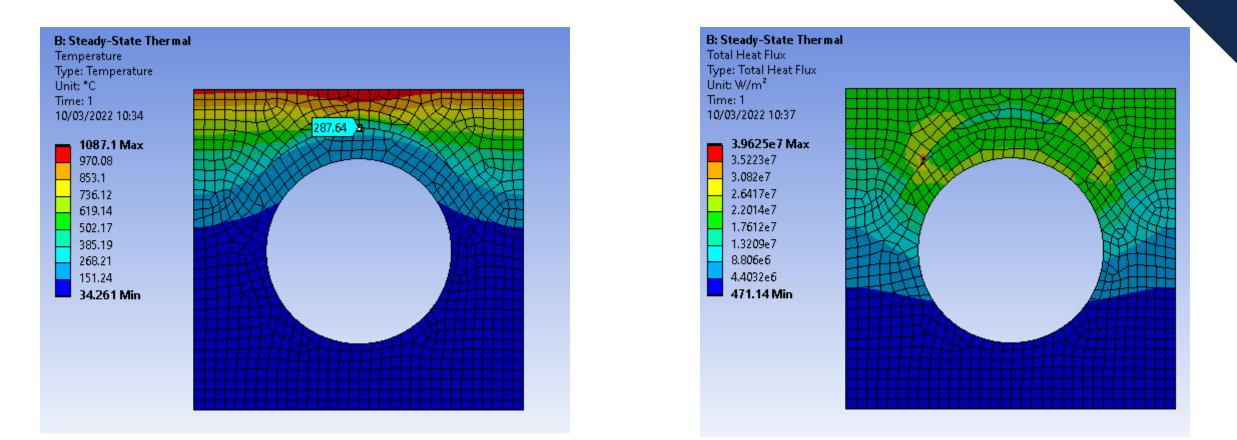
At incident heat flux of 20MW/m<sup>2</sup> results in a CHF margin of 1.44
