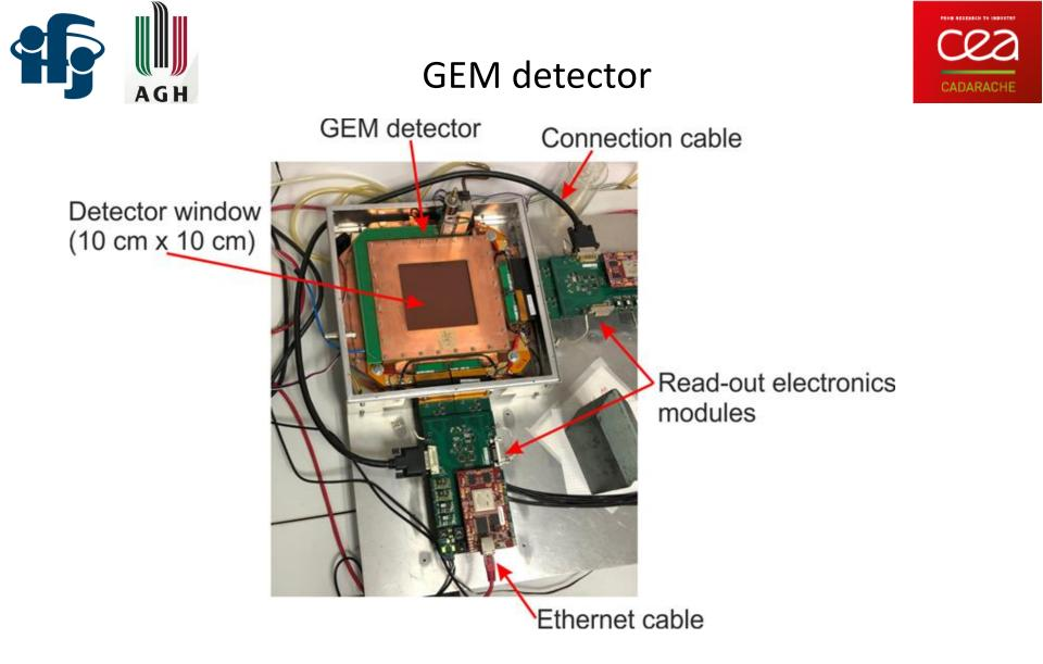
The GEM detector developed at the laboratory of Nuclear Electronics and Radiation Detection Group
