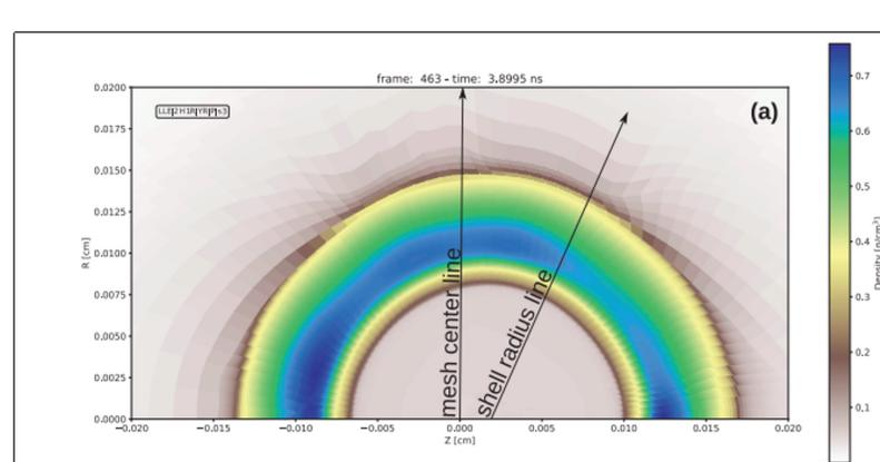
2D density map of a dynamic shell target near stagnation, in a case with a pre-imposed low mode asymmetry
