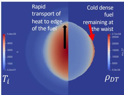
Hotspot thermal conduction suppressed along waist leading to elongated hotspot
