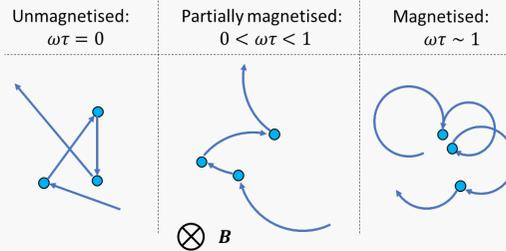
Magnetization *reduces thermal conduction losses from the hotspot.*
