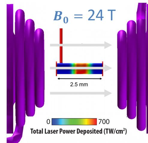
Laser drive: 40 UV beams, 1.5 ns, total energy of 14.5 kJ,  $> 5 \times 10^{14}$  W/cm<sup>2</sup> across 650  $\mu\text{m}$
