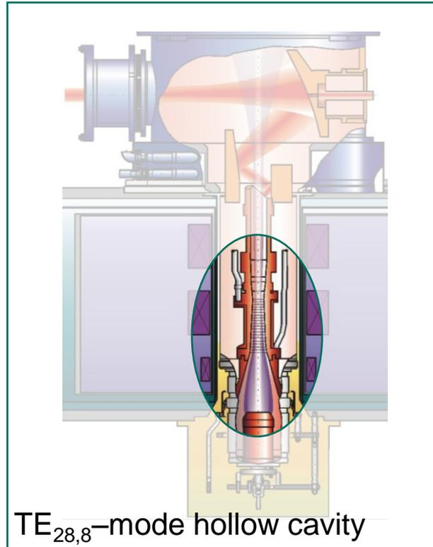
TE<sub>28,8</sub>-mode hollow cavity
