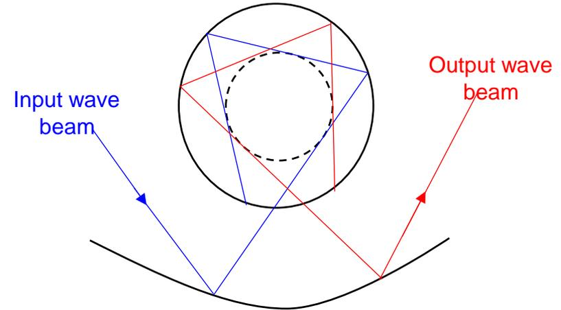
**Launcher for co- and counter-rotation operating modes used for phase locking operation.**
