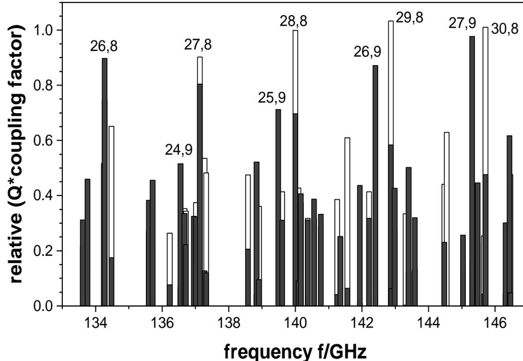
**Very dense mode spectrum even for 140 GHz TE<sub>28,8</sub>-mode gyrotron.**
