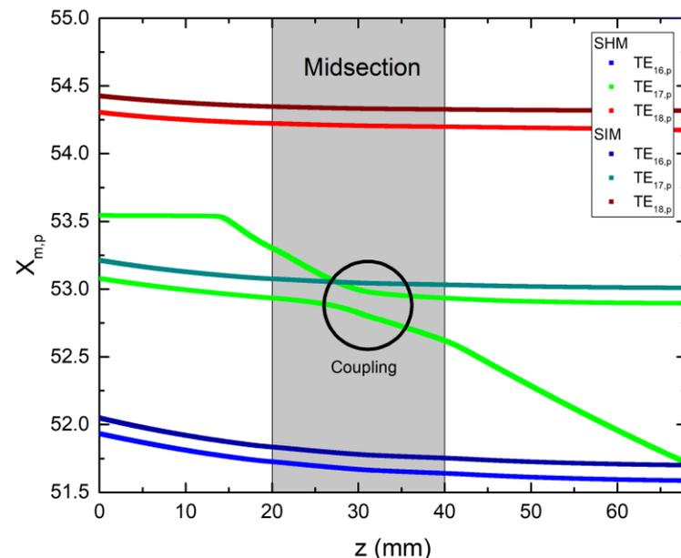
Comparison of eigenvalue spectrums versus  $z$ , without (SIM) and with (SHM)  $N=27$  outer corrugations
