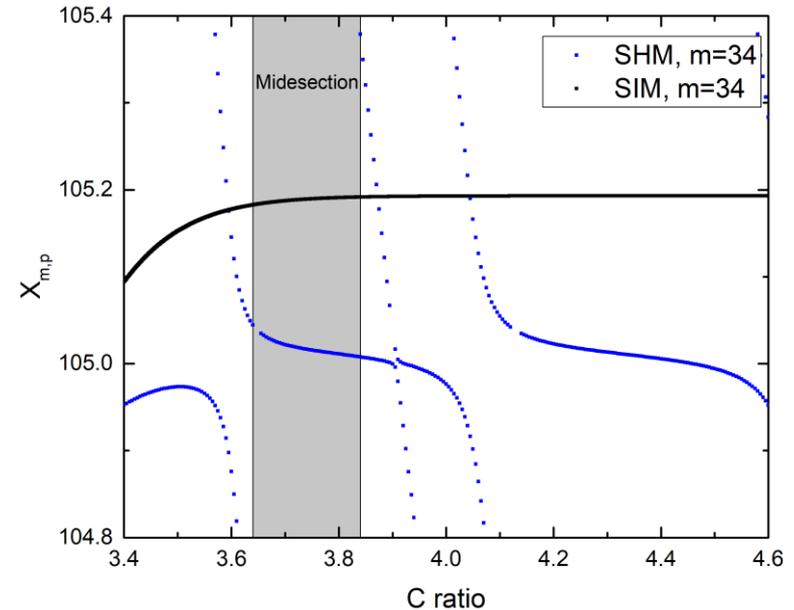
Comparison of eigenvalue spectra versus  $z$ , without (SIM) and with (SHM)  $N=27$  outer corrugations for  $TE_{34,19}$ .
