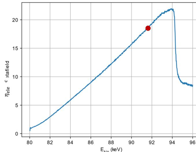
**Limitation: thermal loading on inner conductor (230 W/cm<sup>2</sup> / red dot)**
