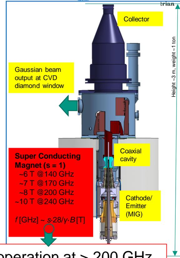
The required magnetic field becomes an issue for operation at > 200 GHz
