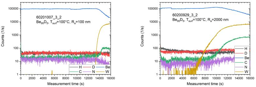
Example: SIMS depth profiles from two otherwise similar Be samples with different roughness
