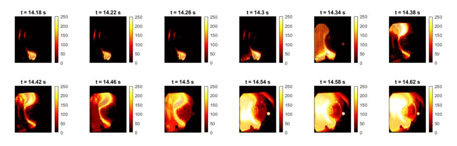
We are developing a simple and fast algorithm to detect anomalous VIS radiation, track and characterise it.
