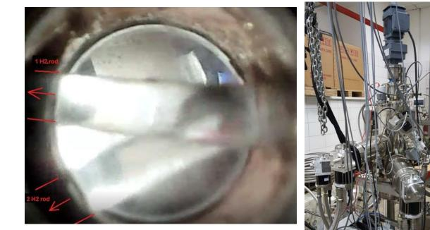
Two ice rods for higher throughput Still some issues with timing of pellet delivery to be addressed
