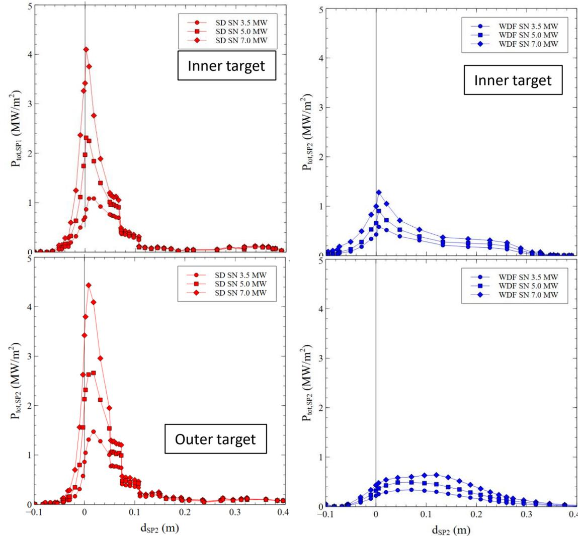
In pure D with the wide divertor detachment is obtained below  $P_{SOL} \approx 7$  MW at  $n_{sep} = 7 \cdot 10^9$  m<sup>-3</sup>
