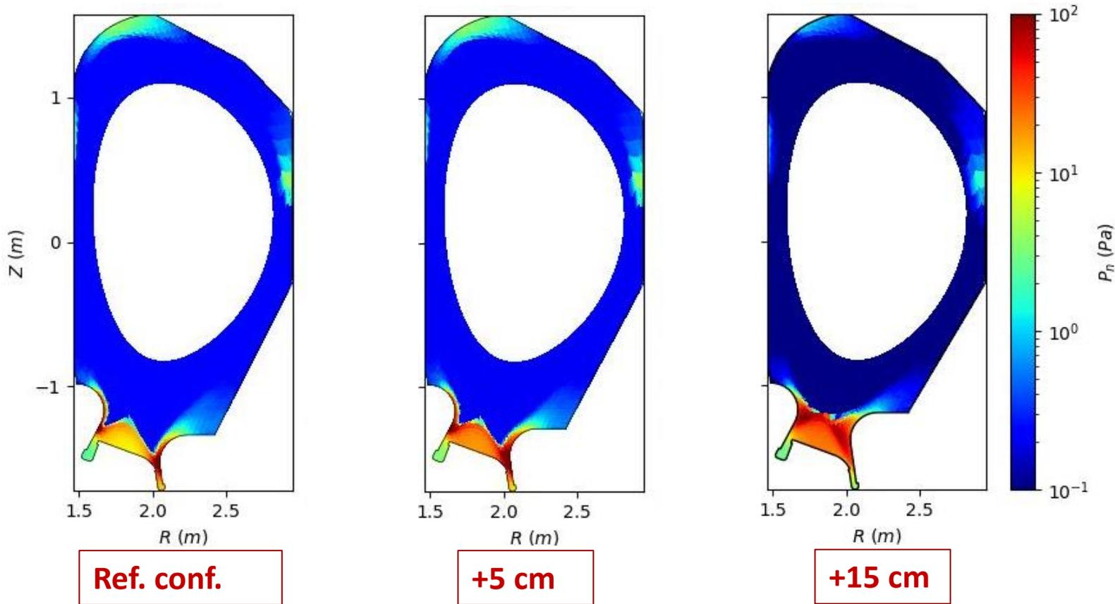
Increasing outer target length will reduce neutrals pressure outside the divertor
