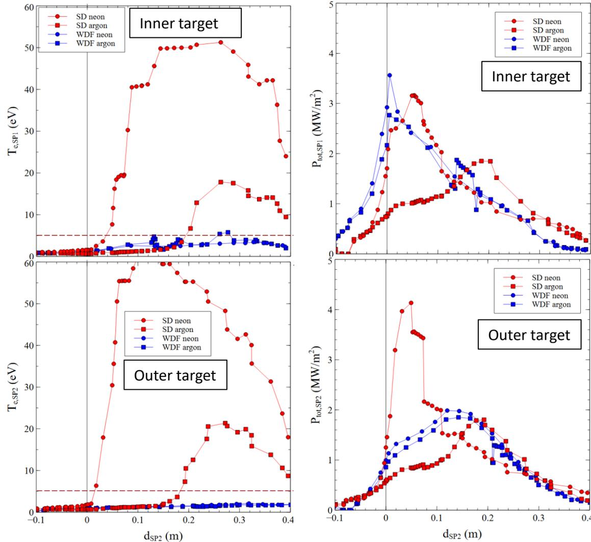
**Lower target temperature with wide divertor at both targets**
