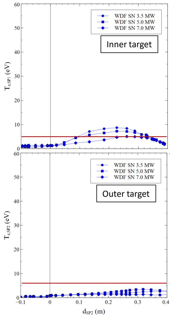
In pure D with the wide divertor detachment is obtained below  $P_{\text{SOL}} \approx 7 \text{ MW}$  at  $n_{\text{sep}} = 7 \cdot 10^9 \text{ m}^{-3}$
