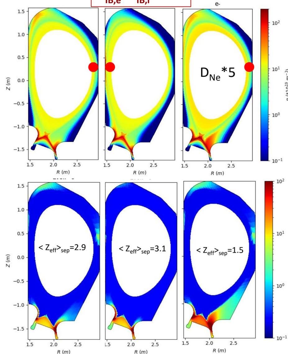
Tested different gas-puffing locations, equal  $P_{IB}$  splitting between electron and ions, higher impurity transport or lower divertor transport
