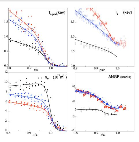
$I_p = 2.5 \text{MA}, \ B_T = 2.7 \text{T}, \ q_{95} = 3.3, \\ \delta_u = 0.4, \ \text{VV}, \ \text{D-gas} = 3.5 \ \text{x} 10^{22} \ \text{el/s}. \\ P_{\text{IN}} = 32\text{-}34 \text{MW}$
