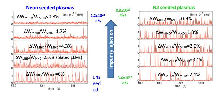
The ELMs are very different between Ne and N-seeded plasmas as the impurity seeding rate increases.
