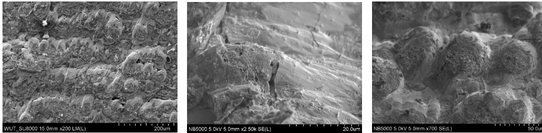
SEM images of the deposit morphology, sample J.
