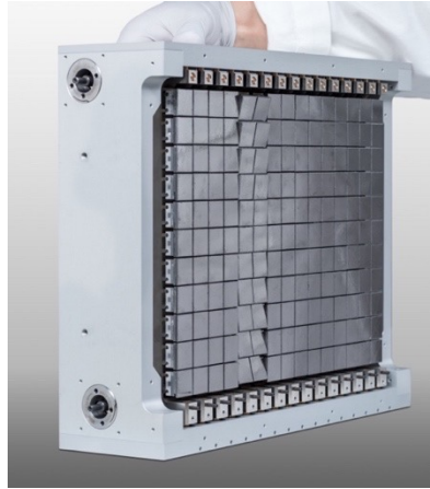
HOPG monochromator Effective Area 300 x 165 mm 2 cold and thermal neutrons flux : 10^9 n/cm 2 /s at (at 1.5 Å)
