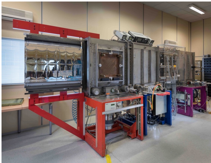
Sputtering machine (ILL) - Production 0.8 m 2 / day
