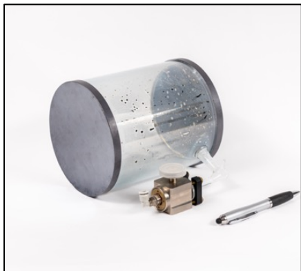
Glass cell with Si windows (Small angle neutron scattering)
