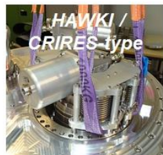
Anti-vibration (AV) mounts for compressors (left), coldheads (middle), Helium lines (right)
