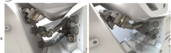
Divertor RH connector under triangular support in disconnected (left) and connected (right) positions
