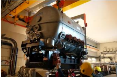
The Beam Combiner Instrument during installation into the VLT laboratory.
