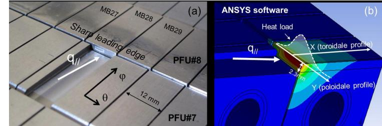
MEMENTO simulations of the first experiment: Melt volume exsibits high sensitivity to small power variations
