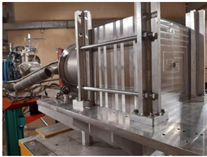
W–shield assembly at ENEA–FNG
