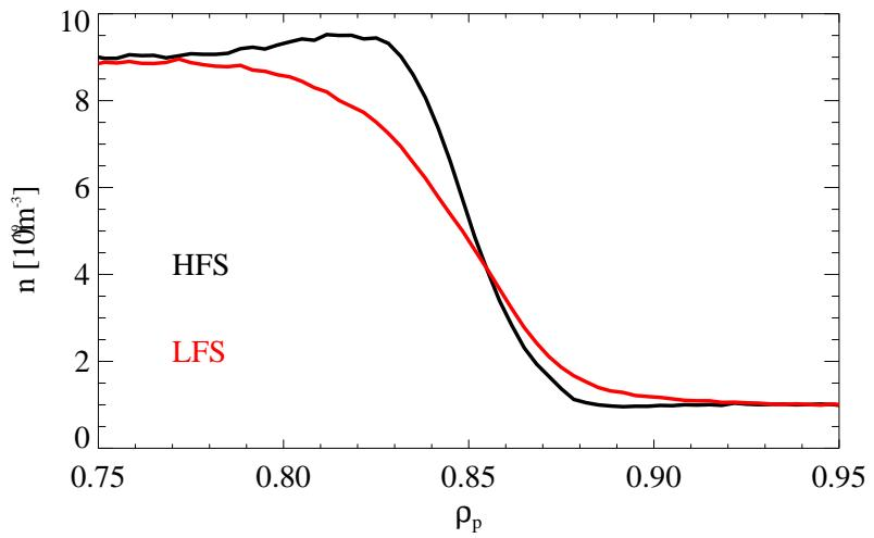
The poloidal density variation is different from that caused by the centrifugal force
