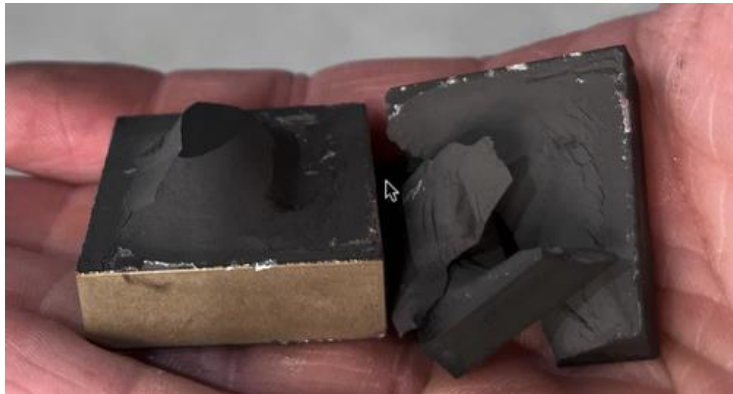
Destructive testing => 120 Nm
