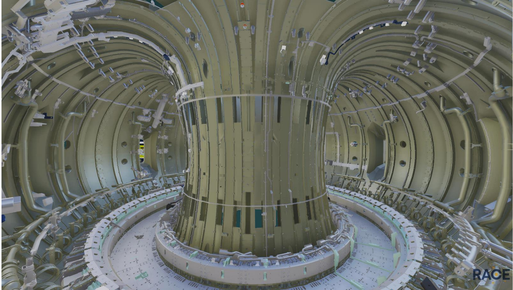
Items removed in phase 2.2 – Saddle Coil Bars (All IL, OL, OU), Restraining Ring.
