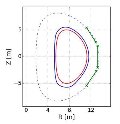
Solid – plasma boundary Solid – resistive wall (~first wall) Dashed -- auxiliary coil surface X- coil positions (geometric)
