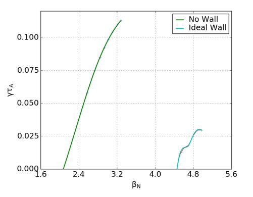
Stability limits for the pressure-driven external kink calculated by pressure scans
