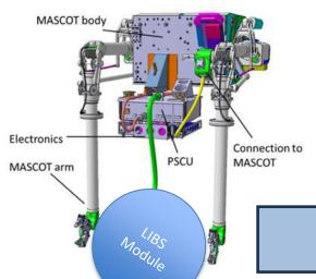
MASCOT has recently been used for deploying a prototypal LIBS tool inside the JET mock-up, where a dedicated mechanical support has been designed and realized with attachment points to allow the MASCOT arms to grip the tool.
