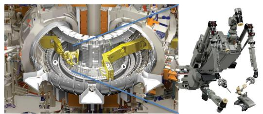
The MASCOT telemanipulator robot is a twoarmed machine with back-drivable actuators and a large dexterous workspace in which each arm can operate within the full 6 degrees of freedom. The manipulator is remotely operated from a control room, where a kinematically similar master manipulator is used to control motions, and provide high-fidelity force feedback
