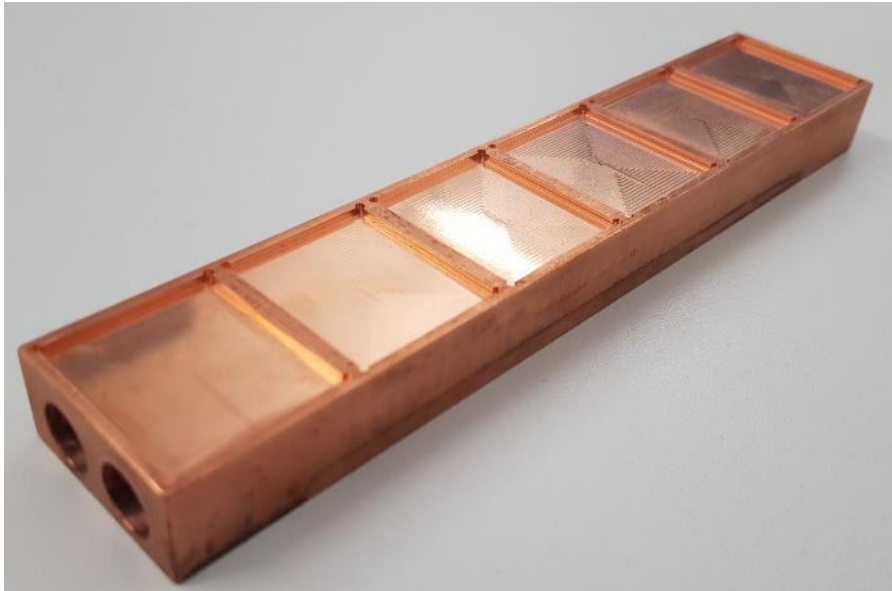
Cu-cooling structure fitting JUDITH 2 clamping
