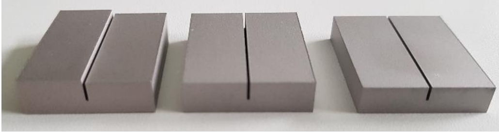
W-tiles: „monoblock pair“, 8 (reference) or 7 mm thick (for deposition)
