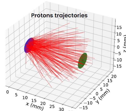
3D view of proton trajectories generated from the PET foil toward the Si detector
