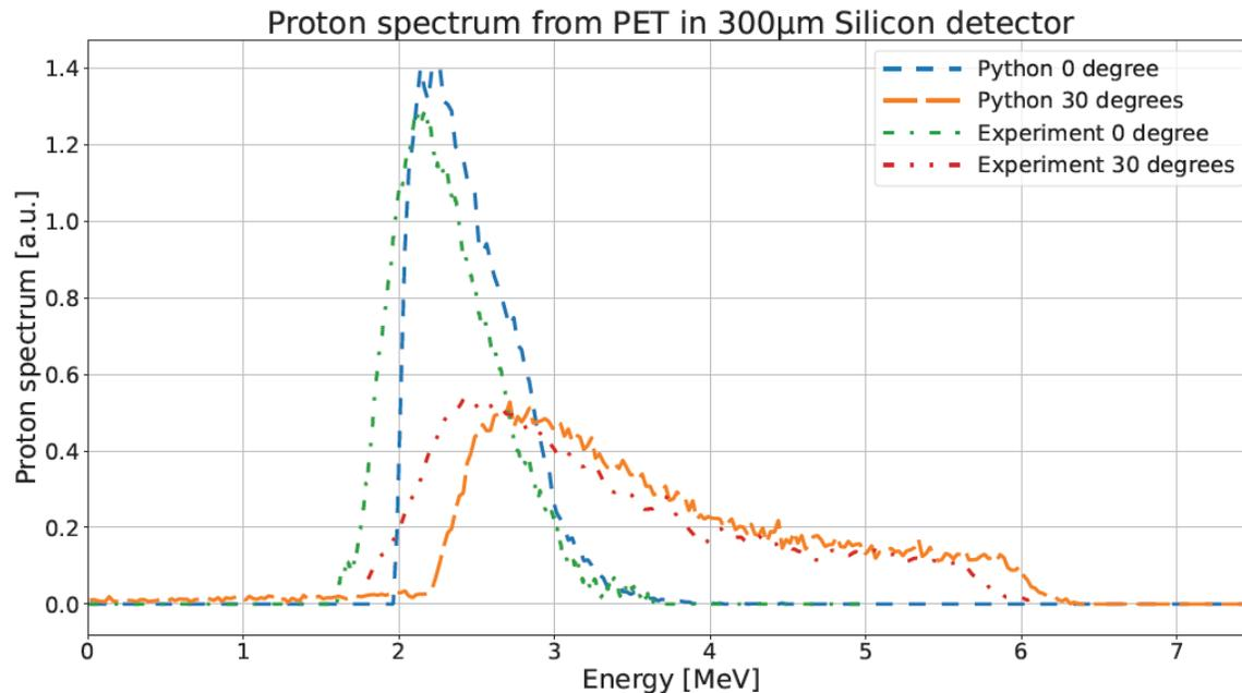
A good agreement is observed between the simulations and the experiment, both in terms of shape of the spectrum and peak location, for the two angles investigated
