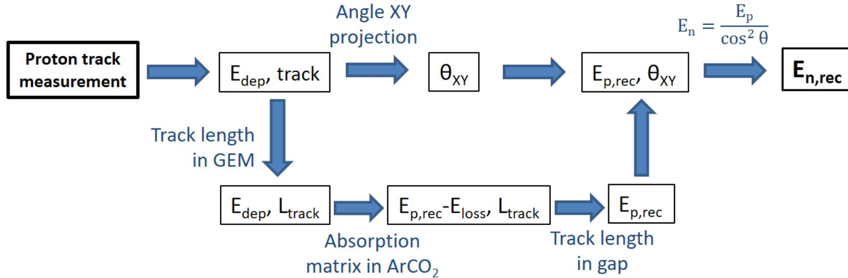
Methodology to reconstruct the incident neutron energy  $E_{n,rec}$  based on the measured proton tracks in the NS-GEM prototype, where
