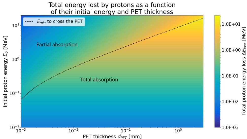
Absorption matrix of proton energy  $\Delta E_{loss} = f(E_0, d_{PET})$  in PET
