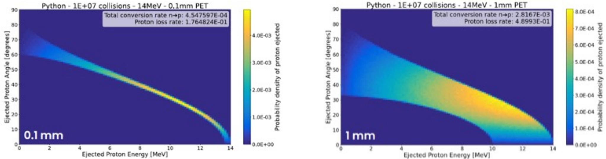
As an example, such distribution obtained with this simplified model for 14 MeV neutrons and PET thicknesses of 0.1 mm and 1.0 mm are presented in above fig.
