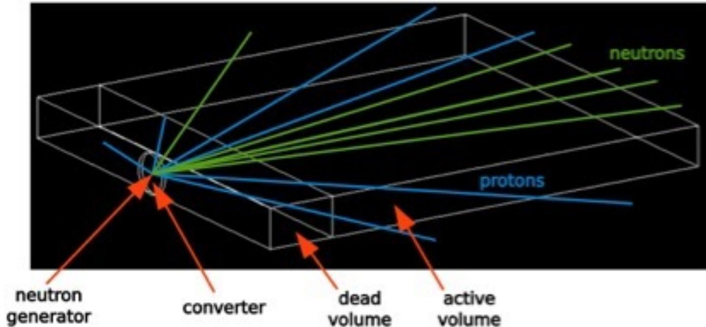
A sketch of the detector model created in the GEANT4 software and used for the performed simulations. The developed model consists of: 10 mm diameter circular converter with variable thickness, neutron generator placed in the centre of the converter and two separate cuboid-shaped active ( $100 \times 100 \times 10 \text{ mm}^3$ ) and dead ( $17 \times 100 \times 10 \text{ mm}^3$ ) detector volumes.
