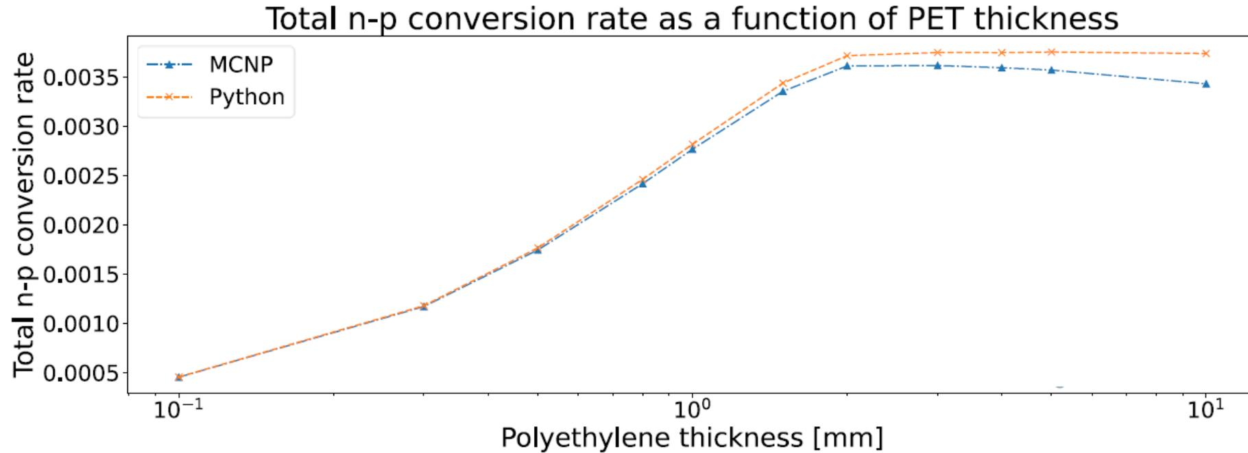
Benchmark of the obtained total n-p conversion rate against MCNP, as a function of the PET thickness. The maximum possible conversion rate is  $3.77 \cdot 10^{-3}$ .
