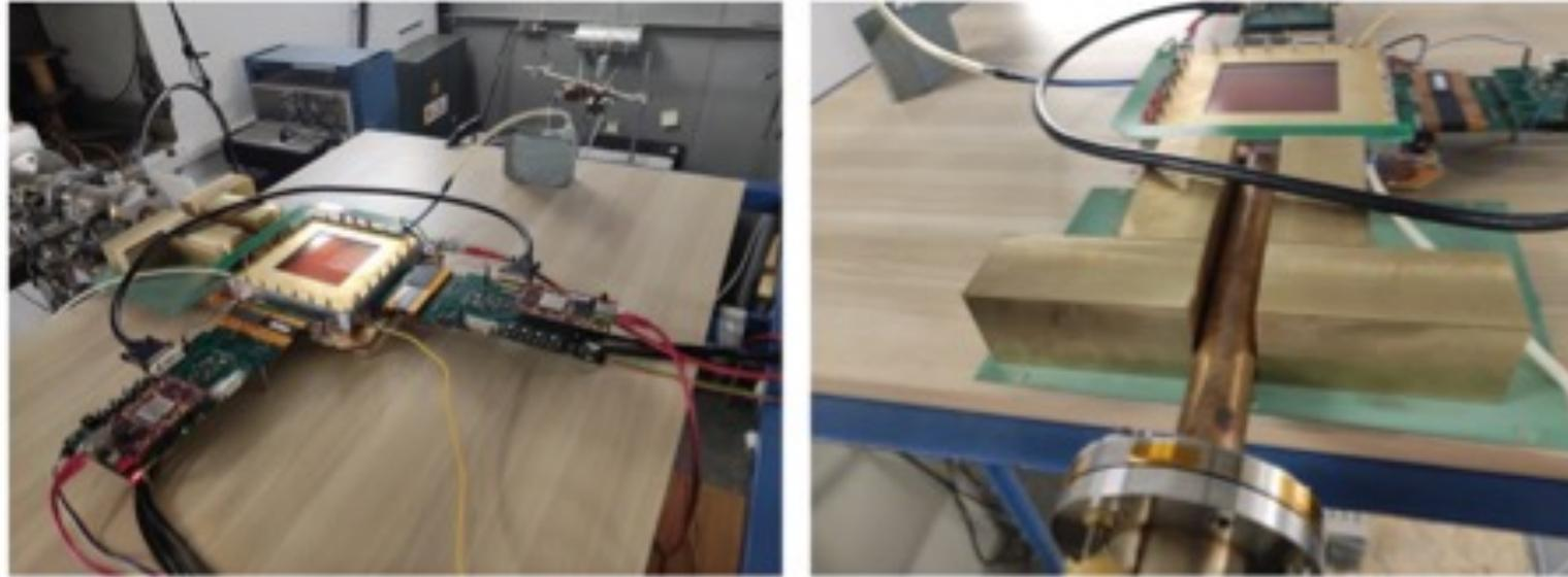
For performed tests 25 cm collimator and 0.5 mm converter has been used. Data have been collected for 3 hours in 15 minutes periods.
