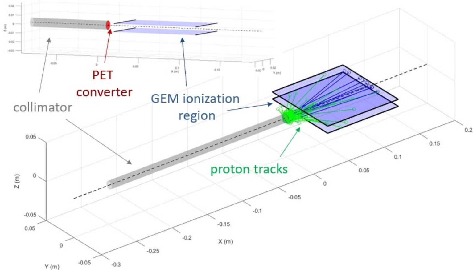
3D view of the NS-GEM model used in matlab simulations, with the collimator in grey, the PET converter in red, the two GEM planes defining the gas ionization region in blue, and several proton tracks in blue (reaching the GEM back plane) and green (stopped before reaching it)
