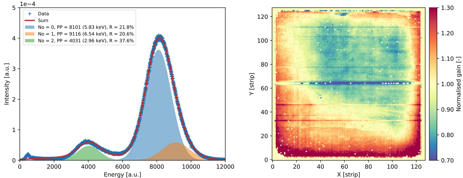
Performed tests confirmed stable operation of the detector and its performance as expected. The obtained energy spectrum and gas gain factor distribution map are shown in Figure (left and right respectively). The energy resolution is around 22% FWHM for the 5.9 keV line.
