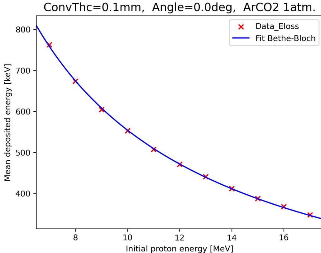
dE/dx calibration curve generated for 0.1 mm converter, scattering angle 0 deg, protons detected at 0 deg, and ArCO2 70/30 gas mixture at 1 atm. pressure
