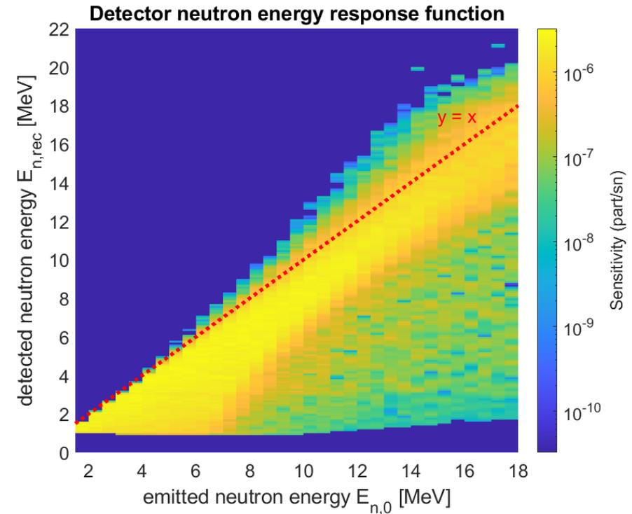
The theoretical energy response function of the NS-GEM prototype is determined, for the 0.5 mm PET (thickness used experimentally), by repeating the procedure for several neutron incident energies from 1.5 MeV up to 18 MeV, by steps of 0.5 MeV. The resulting matrix is presented both in linear and logarithmic scale.
