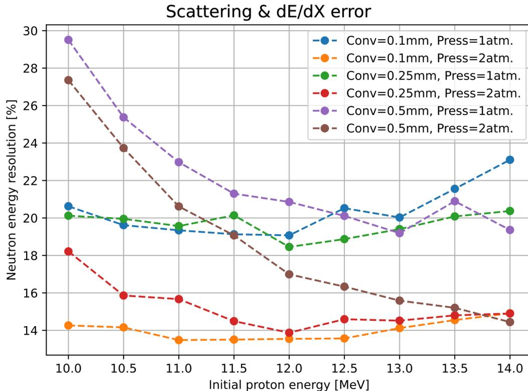
Summary of energy resolution of reconstructed neutron energy taking into account both scattering and specific energy losses dE/dx for three different thicknesses of the converter and ArCO<sub>2</sub> 70/30 gas mixture at two different pressures.
