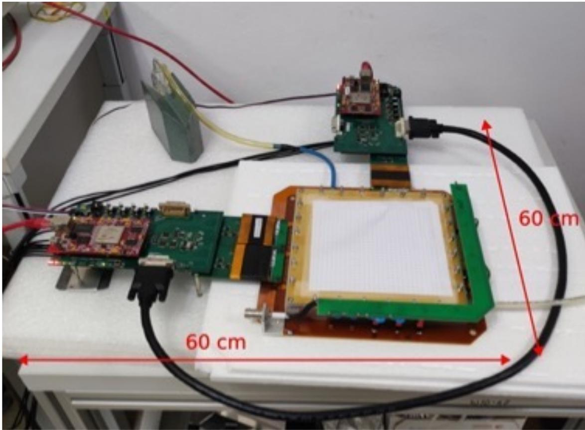
The assembled NS-GEM detector has been first tested extensively using X-ray  $^{55}\text{Fe}$  radioactive source following our standard test and calibration procedures.
