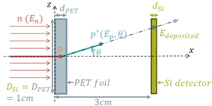
Parametrization of proton trajectories, including a Si detector placed 3 cm behind the PET foil
