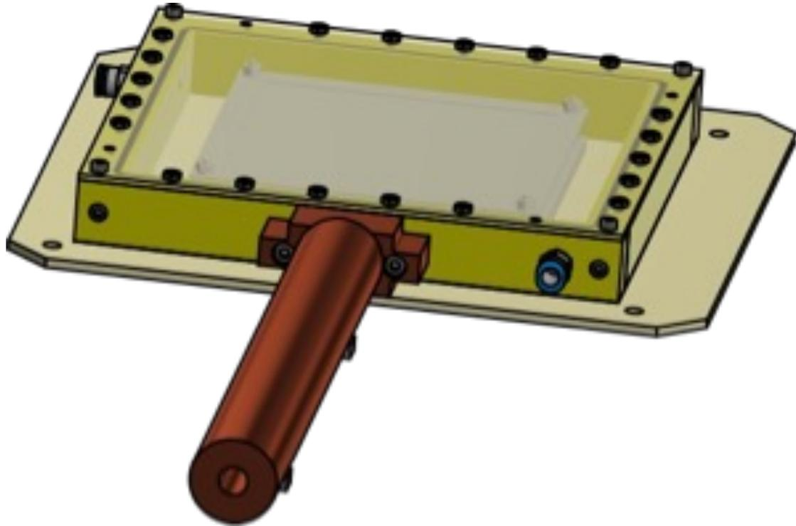
As proposed in the initial phase of this project our demonstrator detector is based on a standard 3-stage GEM detector, however, with the thickness of drift region enlarged up to 10 mm compared to the standard thickness of 3 mm. This modification required designing and manufacturing of a new detector frame and proper modification of the voltage divider to ensure the same level of the electric field in the drift region as in the standard design.
