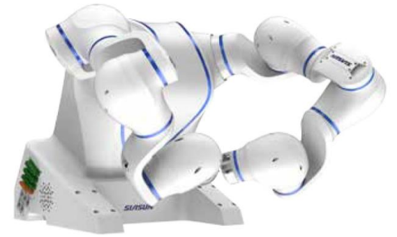
Flexible dual arm Payload: 25 kg Repeatability: ± 1 mm
