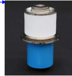
DPA tube prototype testing , 100kW,1000s
