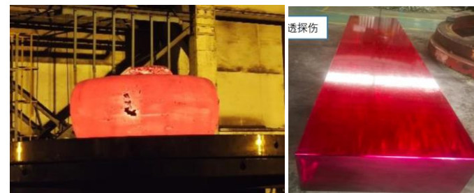
Forging 1-10T ESR ingot
