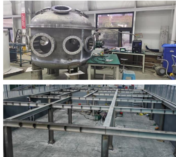
Vacuum chambers and supporting structure
