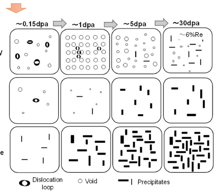
**Displacement defects + Transmutations elements**
