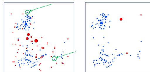
Primary damage      After annealing
