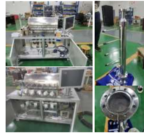
Pebble bed gas pressure drop testing
