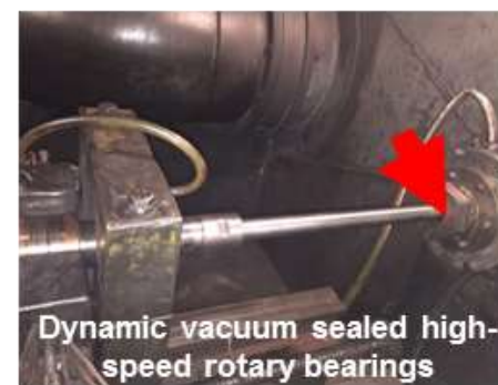
Fabrication of Be pebbles based on rotating electrode method
