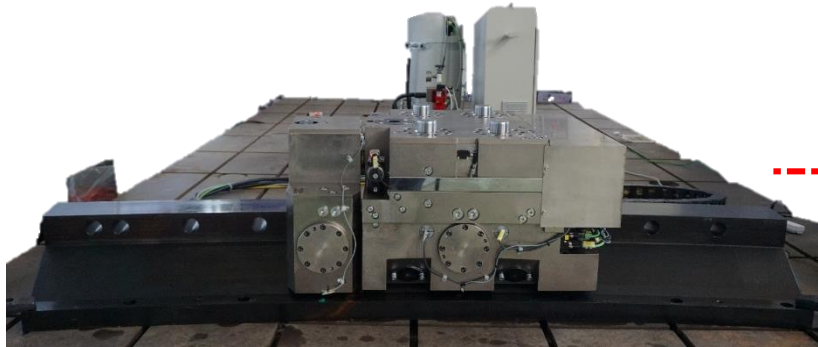
Blanket toroidal Mover system, repositioning accuracy \pm 1 mm. Two mover system finish the functional test in June 2023.
