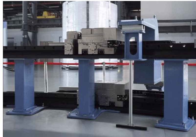
Dual Mover motion synchronization test facility
