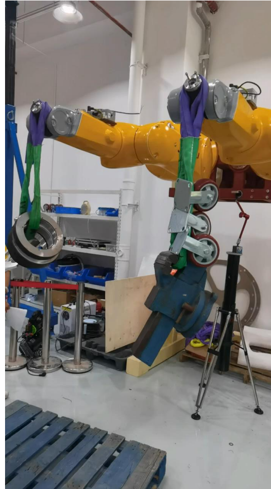
Load and deformation testing
