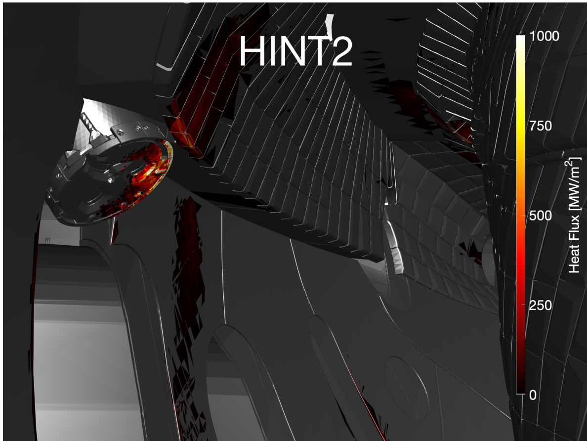
Figure 9. Fast ion wall loads for a synthetic view from the fast ion wall load monitor diagnostic. The HINT2 simulation results are shown.
