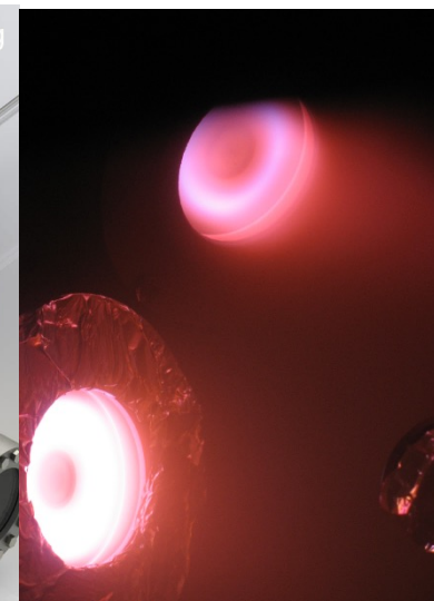
Ignited W and Be MS plasmas under D/Ar atmosphere
