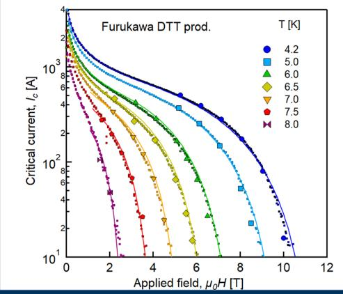
Results of transport (markers) and magnetization measurements (small square symbols) at several temperatures versus the applied magnetic field. Lines represent the fit to the *two-component model* for the NbTi critical surface.
