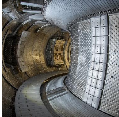
W-coated C PFUs + 14 bulk W PFUs
