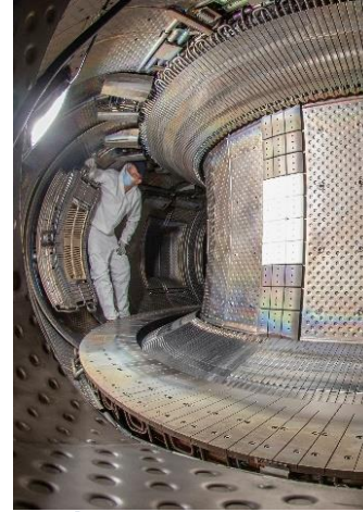
W-coated C PFUs + 56 bulk W PFUs BN tiles on inner bumpers
