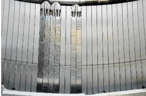
W-coated C PFUs + 5 bulk W PFUs
