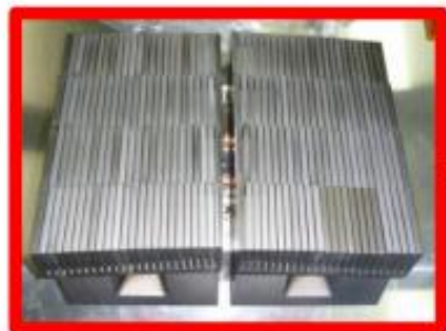
Bulk tungsten (W) Lamellae structure
