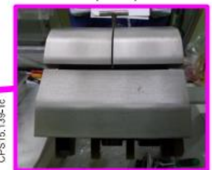
Tungsten (W) coating on carbon-fibre composite (CFC)
