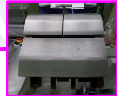
Tungsten (W) coating on carbon-fibre composite (CFC) tile
