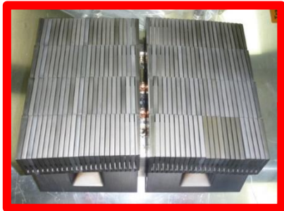
Bulk tungsten (W) Lamellae structure
