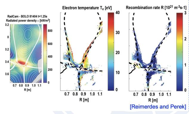
2D Te map from MANTIS diagnostic with significant signature of recombination at inner X-point
