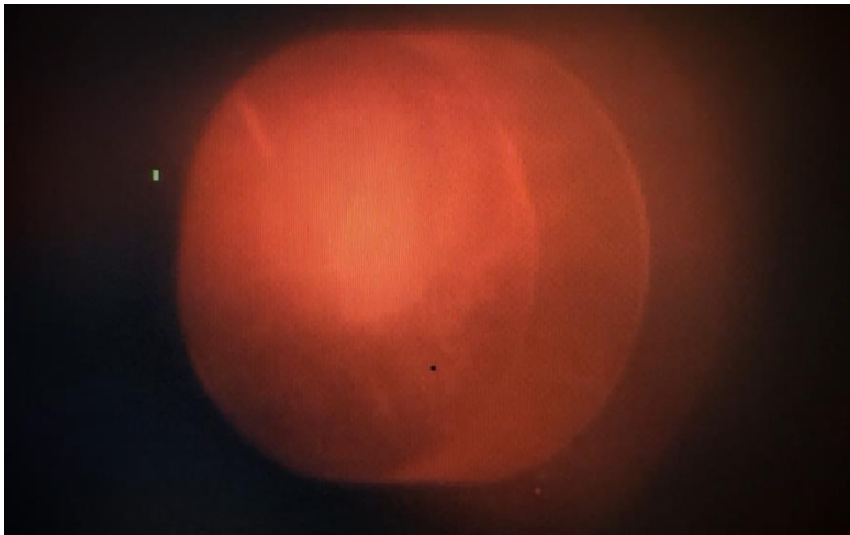
Fast IR capture of W target during exposure (left), post-exposure LOM micrograph (right)
