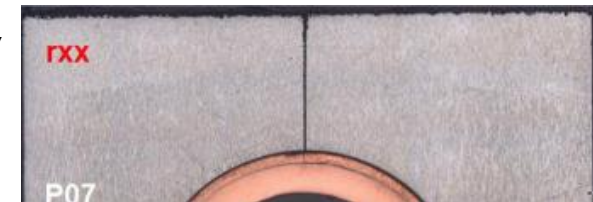
Deep cracking of a W monoblock after 300 cycles of 20 MW m -2 (M. Li et. al, 2015)
