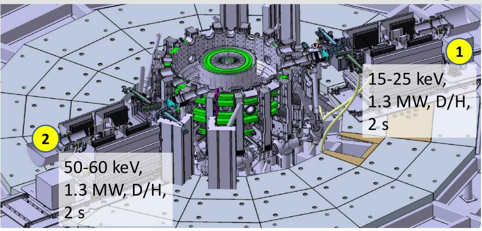
Limitations are currently in place: only 1.1 MW for NBI-2, max injected energy 1.7 MJ for NBI-1 and 2 MJ for NBI-2. Work is underway to permit relaxing these limitations.
