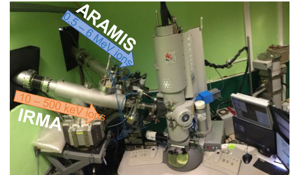
In situ TEM coupled to 190 kV IRMA ion implanter and 2 MV ARAMIS accelerator
