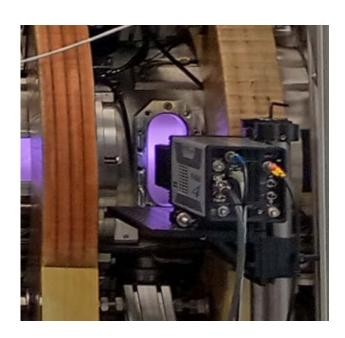
System based on imaging optics, optical filtering and a very short (down to ~1ns) gating time ICCD camera.
