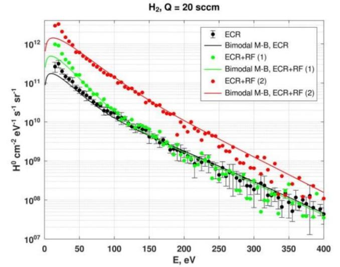
Differential flux spectra of neutrals for ECR and ECR+RF discharges. The experimental data: ECR, ECR+RF (1) for  $P_{RF} \approx 0.26 \text{ kW}$ , ECR+RF (2) for  $P_{RF} \approx 1.57 \text{ kW}$ .
